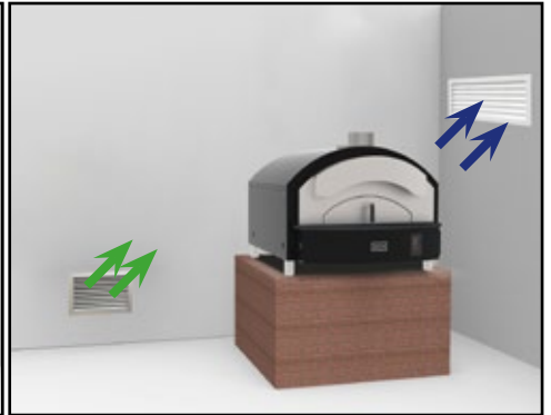
➔ NATURAL VENTILATION - S=300\text{cm}^2 ➔ NATURAL AERATION - S>100\text{cm}^2
